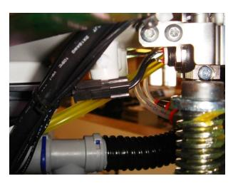
Loosen the two 10 mm. hex nuts which holds the top plate in the rear end.
