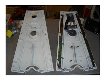
Disassemble the top plate and move the parts to the new top plate. The included part must be used in order to correct the problem with corrosion in cup filler and fountain.
