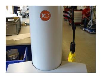
Remove the rear half tube cover AN-955.
