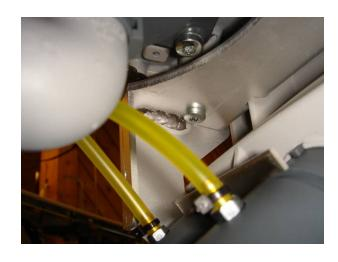
Mount the rear end of the top plate and tighten the two 10 mm hex nuts. Now tighten the two screws in the front end.
