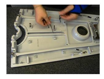
Mount the micro switch for cuspidor flush and the push buttons on top of the top plate.
