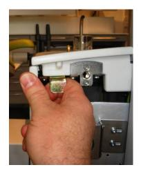
Remove the detachable half tube cover AN-514.
