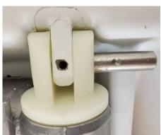
Lift the motor to release it while supporting the backrest. Pull it off the push pull.
