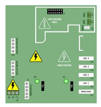
Motor signal connection on "Backplane".
