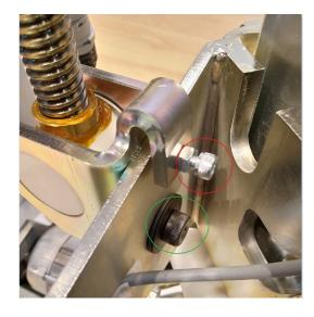
Remove the motor retaining screw located at the base of the chair.
