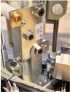
Remove the Motor Protection Cover to gain access to the 3 screws securing the motor to the base.
