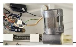
Ensure not to put pressure on the push pull when resting on the base while fixing the new motor. Caution: Always support the backrest when sliding the 4 guiding rods in the push pull.
