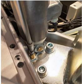
Once the screws are released, lift and replace the motor.
