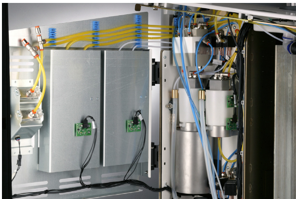
Figure 27 Access to amalgam-separator
