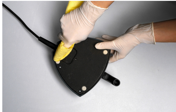
Figure 33 Cleaning of rubber feet
