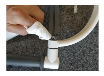
Try turning the arc using the handles. If the friction is too high compared to before, and you can see the sides of the arc has contact to the outer arc, you may remove the arc again and gently file the sides.
