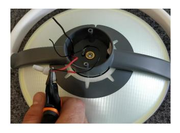
Loosen the bolt in the top holding the light unit.
