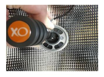
Take note of which side of the light unit the guide is positioned. During reassembly of the new arc, the guide needs to be positioned in the same side as before. If not, the XO Logo will be upside down.
