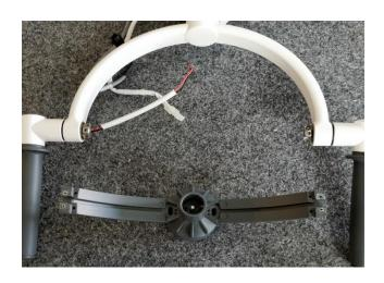
Fit the new arc. It may be necessary to pull the outer arc apart a little bit.
