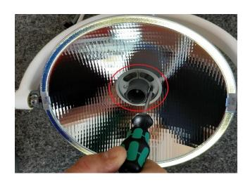
Remove the reflector fixation in each side.
