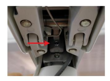
Remove the splash screen by removing the splash screen fixation in each side.
