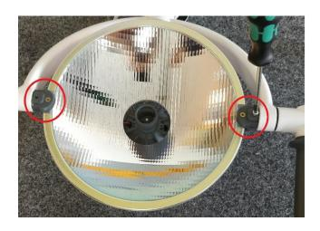
Fit the new supplied O-ring onto the aluminum centre ring and fit the centre ring onto the reflector.
