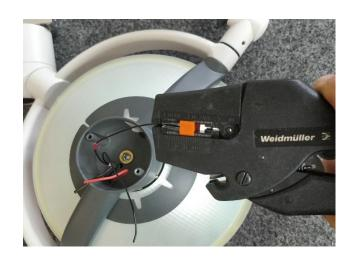
Connect the wires with the splicing terminals.
