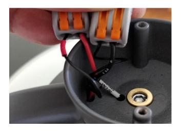
Position the connectors opposite of each other and pull the cable protection over the connectors as illustrated.
