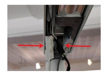
Fit the covers on the underside of the OP Light arm.
