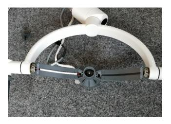
Remove the two plastic parts in each side of the arc.
