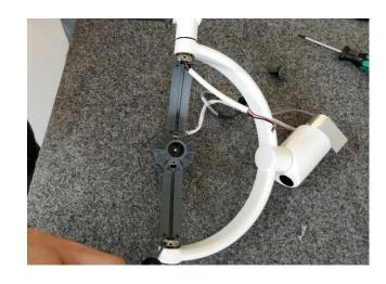
Remove the 4 screws from each side of the arc.
