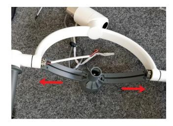
Use the supplied Loctite on the four bolts for the arc.
