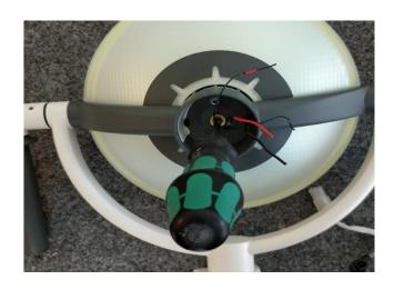
Carefully pull out the light unit from the light head.
