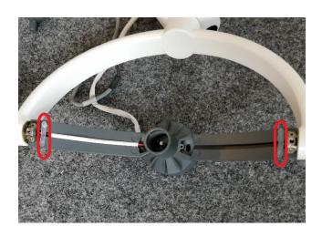
Remove the wires from the arc.
