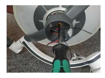
Adjust the distance of the light unit with the screw in the top, to match the measurements/marks made earlier during disassembly.
