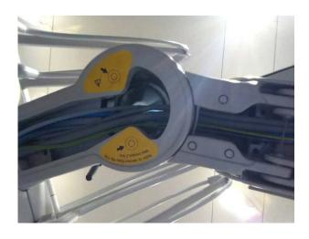
Draw the cable together with the other cables in the bridge arm.
