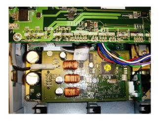
Mount the special MX2 micromotor power supply (AO-136) inside the unit stand as shown, with the enclosed screws.
