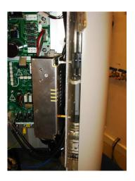
Connect cable CA-073 marked "DMX Power" to the MX power supply.
