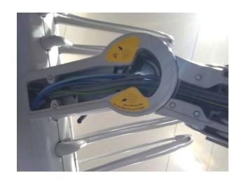
Mount the MX2 valve module in the bridge at the preferred instrument position.
