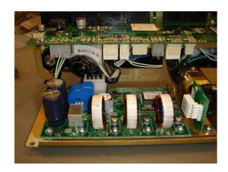
Mount the cable CA-073 in the arm by removing the covers on the underside of the bridge arm.
