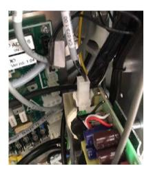
Connect the 230VAC power plug to an unused AUX plug on Mains PCB. (J11, J12, J13 or J14)
