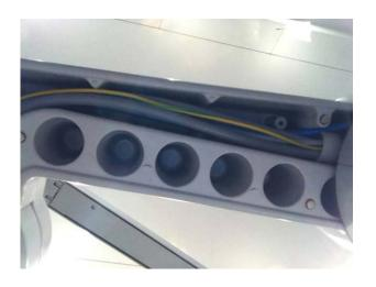
Place the cable together with the other cables in the bridge arm, starting from the unit stand.
