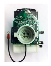
If necessary mount the new Power driver PCB and remember to connect the cables on the PCB before mounting the 5 screws that holds the PCB.
