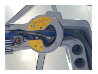
Draw the cable together with the other cables in the bridge arm.
