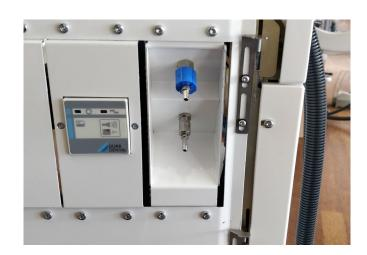
Connect the supplied 4mm air and water hose to the quick connectors.
