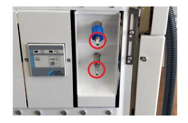
Be sure to remove the couplings before switching on the unit.
