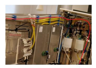
Cut the 4mm water hose to desired length, and connect the water hose to the T-connector on the water regulator.
