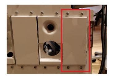
Fit the new panel with the quick connections on the service hatch.
