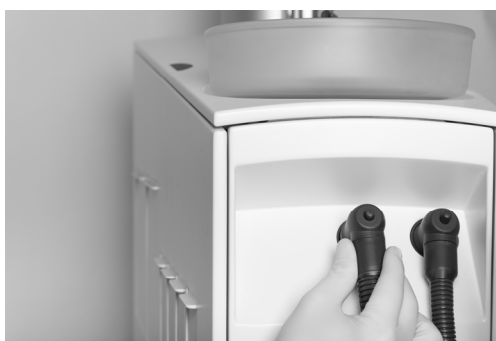
Figure 70 – Removal of suction hoses and filters
