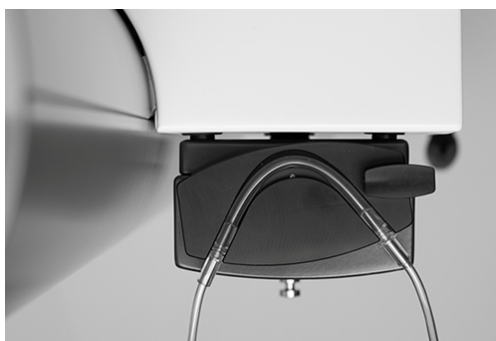
Figure 31 – Attaching the irrigation tubing
