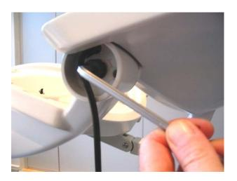
5. Pick the new MG-783 Threaded bushing from the kit and add Loctite 243 (UH-053) to the front part of the thread, before fitting.
