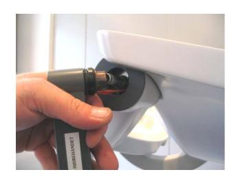
16. Tighten the hexagonal screw to obtain a suitable tension and friction for the arm movements.
