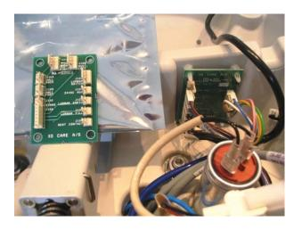
21. Wires and air hose fitted to cable holder with cable binders.
