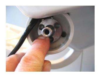
7. Drill the 3 holes using an ø3.3 mm drill to a depth of min. 15 mm. It may be a good idea to drill one hole, cut the thread and fit the first screw. Then drill the other 2 holes, whilst the spindle is held in the correct position.
