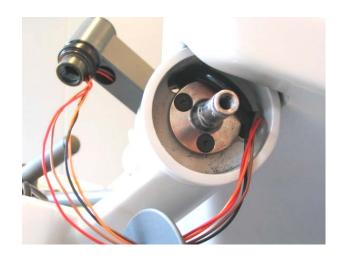
15. Fit the cover over the hole and press the arm onto the spindle.
