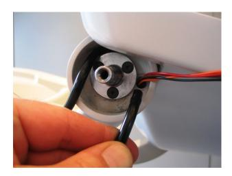
14. Carefully pull the wires (and air hose) through the hole until the suction hose holder can be fitted on the spindle.
