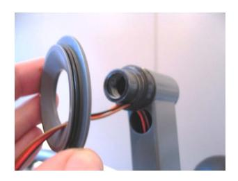
12. Pull the 4 wires from the suction hose holder out through the hole. Make sure the wires take up as little space as possible to leave room for the air hose of the lumbar support, if present.
