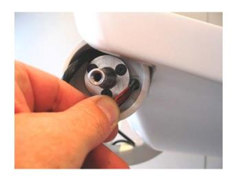
13. If the lumbar support is fitted, lead the air hose through the same hole as the wires.
