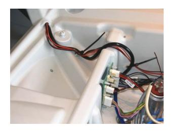
22. Connect the cable from the suction hose holder to J108 "Suct. Left" or to J109 "Suct. Right", depending on type.
