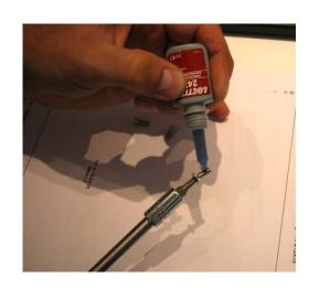
10. Mount the spindle with the screws supplied. Tighten the screws well, with a torque of approximately 1,5 Nm.
