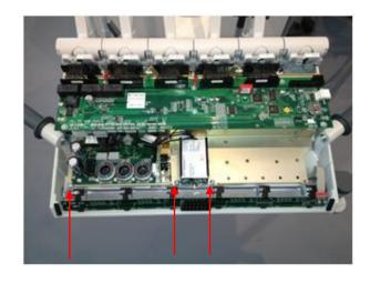
10. Disconnect all air, water and electric connections, and remove the PCB rack.
