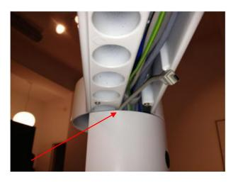
20. Pull the cable trough the rear arm joint.
