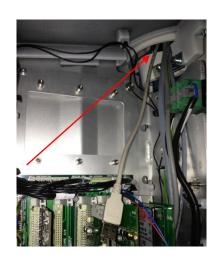
18. Remove the stand cover and pull the cable from the Unit stand to the instrument bridge arm.
