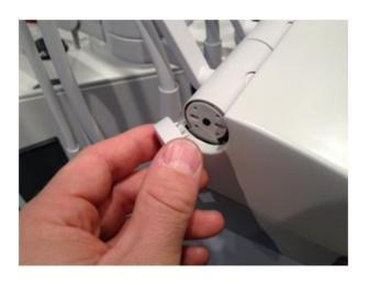
2. Loosen the two torx 20 bolts in the instrument bridge top cover. Remove the top cover.
