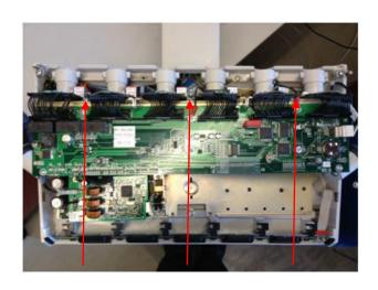
9. Loosen the three PCB rack attachment bolts.
