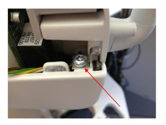
4. Loosen the left hand attachment bolt for the suspension rack.
