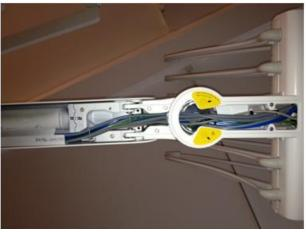
17. Install the cable starting from the Unit stand.
