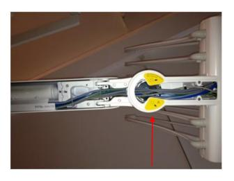
22. Connect the cable to the valve block cable.
