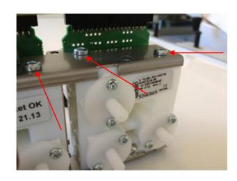
12. Remove the lower attachment bolt from the valve block rack.
