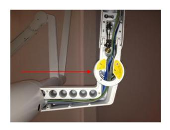
21. Pull the cable trough the forward arm joint.
