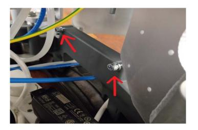
Remove the rear half-pipe panel to access the mounting bracket for the power supply.
