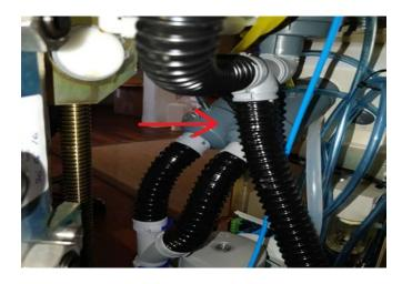
Place the transparent ventilation hose along with the drain hose and secure it with a cable tie.
