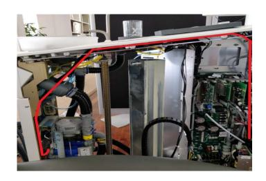
Remove the 4 bolts holding the front panel and remove the panel.
