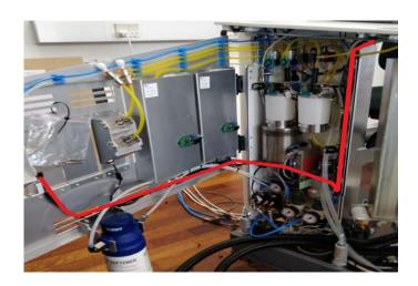
Install the remote-control panel on the service door in 3<sup>rd</sup> position from the left.
