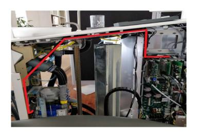
Connect the 2-pin signal cable CA-035 to connector J8.
