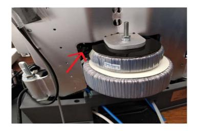
Install the rear half-pipe panel on the unit.
