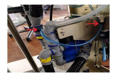
Connect the vacuum hoses for the valves for select vac.
