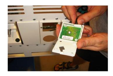
Install the remote-control pad and tie down the cables with cable-ties.
