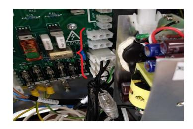
Route the power supply cable for the separator to the separator.
