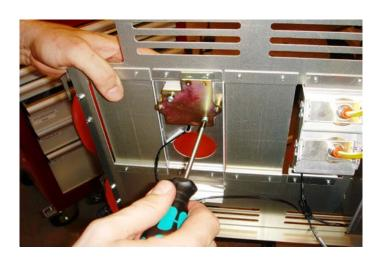
Install the front panel using the 4 bolts and make sure to align the panel by placing spacers/washers the same way as before.
