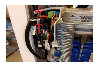
Route the 2-pin signal cable CA-035 to the backplane PCB.
