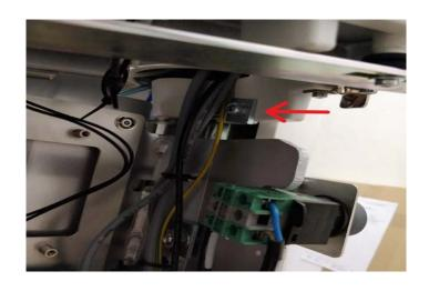
Loosen the 2 bolts holding the rear halfpipe panel at the bottom.
