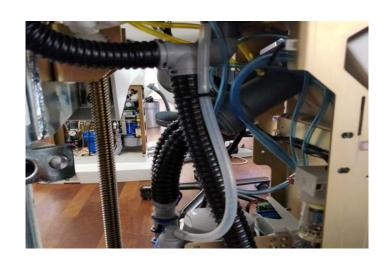
Connect the oil collector drain hose to the fitting found on the tube to select vac.
