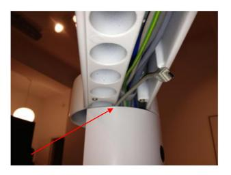
Pull the cable trough the rear arm joint.
