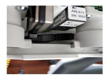
Re-assemble the complete PCB rack in the bridge, and connect all cables and hoses.
