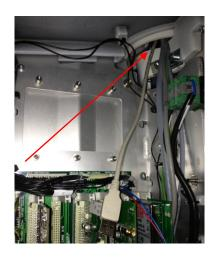
Remove the stand cover and pull the cable from the Unit stand to the instrument bridge arm.
