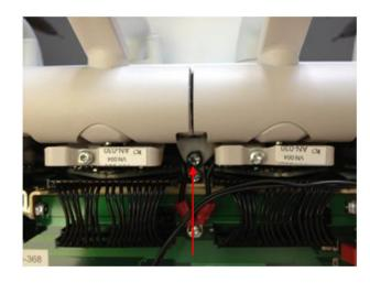
Remove the suspension rack
