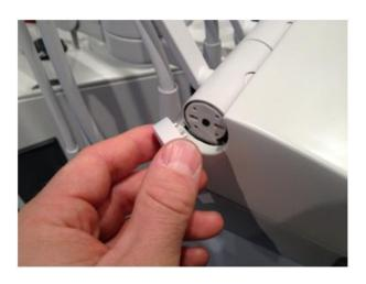
Loosen the two torx-20 bolts in the instrument bridge top cover. Remove the top cover.
