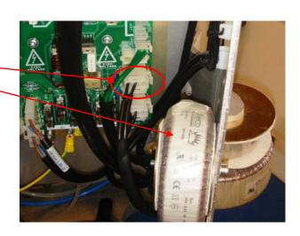
In the top of the backplane find the connecter J8 connect the CA-035 signal cable.
