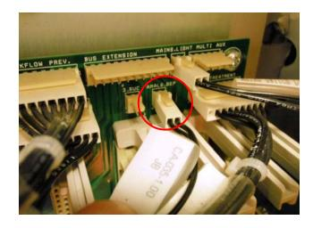
Draw the two cables to the mount-area, located under the select-vac, (Draw together with the other cables under top plate)
