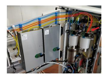
Cut the hoses just above the suction disinfection panel, connect the fittings as illustrated and route the remaining hose from the fittings and down to the suction hose connectors.
