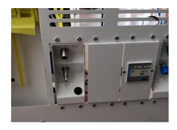
Position the pump V35 as illustrated and secure it with 2 torx20 screws.
