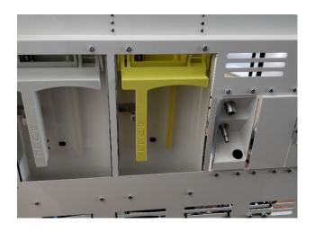
Remove the cover and fit the suction disinfection panel with 4 torx20 screws.
