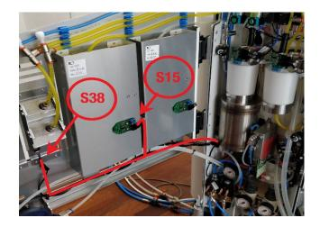
Test the newly installed equipment by running a suction disinfection sequence, and confirm that the system works properly and there are no water leaks.
