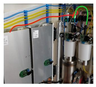
Position the 2 remaining 6mm yellow hoses into the mixing cup and route them to the suction disinfection panel on the service door.
