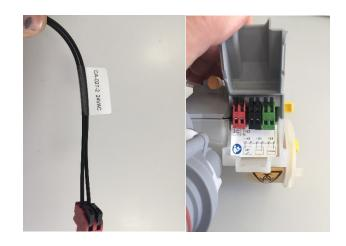
Connect the cable CA-028 to the green connector on the spittoon valve.
