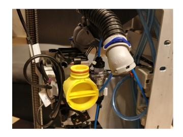
Remove the suction hose connected to the bottom of the spittoon valve.
