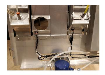
Connect the cable CA-027 to the red connector on the spittoon valve.
