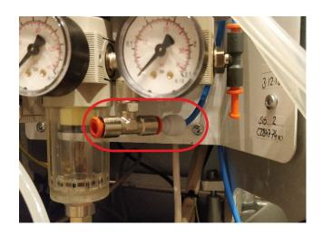
Remove the old 4mm hose for air supply to the spittoon valve.
