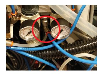
Connect the 6-4 mm reduction fitting to the T-fitting.
