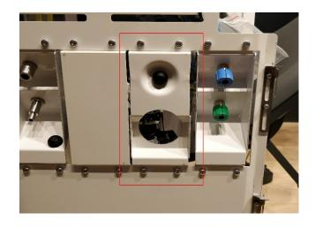
Fit the new spittoon valve panel in the service hatch.
