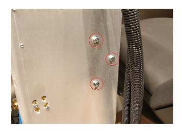
Remove the 2 cable tie holders from the old spittoon valve and mount them on the new spittoon valve.
