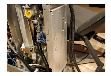
Remove the drain hose from the spittoon connected to the spittoon valve yellow filter.-397
