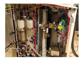
Connect the drain and suction hose on top and bottom of the spittoon valve.
