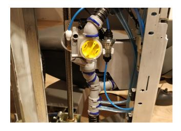
Remove the spittoon valve panel in the service hatch.
