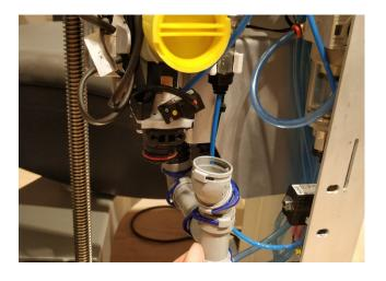
Remove the wires CA-027, CA-028 and CA-098 connected to the panel on the side of the spittoon valve.
