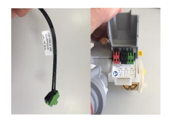
Cut the white connector off cable CA-098 and connect it to the black connector on the spittoon valve.
