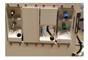
Units manufactured before 1/10-2016: Remove the cable CA-040 (connects the panel on the service hatch to connector X1 on the spittoon valve) and route the supplied cable CA-098 instead.
