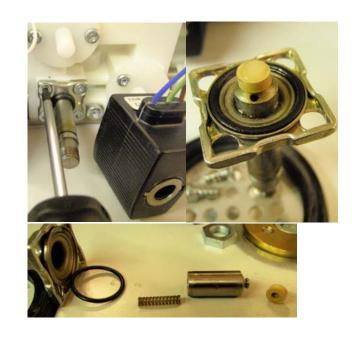
Clean the valve-housing, piston & spring etc. from corrosion, calcium & grease With use of a clean soft tissue. Clean the housing from calcium with use of a calcium dissolver and/or steel wool # 00.
