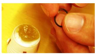
NOTE! X-tighten the screws carefully to make sure the O-ring will make a perfect tight fit.
