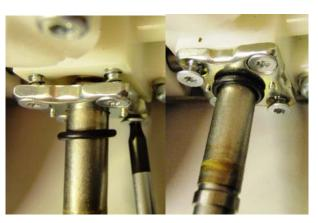
Valve connections to susp. PCB start block.
