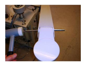
Be careful not to damage the nylon bearings inside the U-profile.
