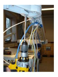
Now you will have to remove the axel holding the U-profile with a cylindrical punch.
