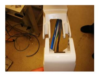
Mount the left axle and put the cables and tubes in, make a loop like shown on the picture and mount the right axle together with the cable holder pin.
