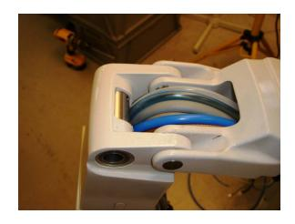
Lift up the forearm link2 and U-profile. Mount the axle removed previously.
