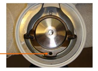
Control the level on the newly mounted lower part by applying a spirit level to the underside as shown on picture. If not in level then level it in according to level instruction of bridge lower part. (YB-797)
