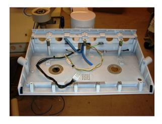
Do not dismount the horizontal locking mechanism from the cable and tube.
