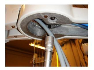
Screw the forearm lower part together with the forearm link2 by using the hex nut and the washer, (NB: use the new one. Supplied in KT-00X Kit).
