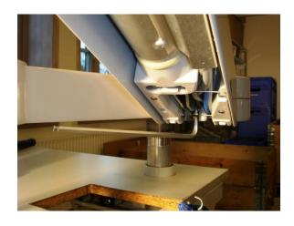
Unscrew the first hex nut which holds the lower part of the bridge.
