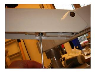
Loosen the balance screw so the arm is not so tight anymore.
