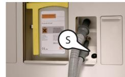
Suction hoses fitted at disinfection nipples.
