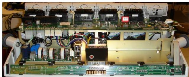
Remove the mounting bracket and mount the included valve module in the position where the dentist wants XO Osseo (Pos. 2 to 6) and re-assemble the valve modules again.
