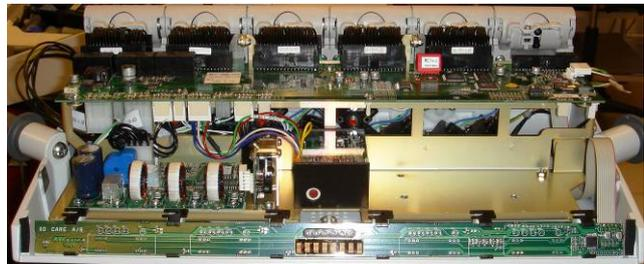
If old Power Driver AN-372 is mounted, then replace it with the included one.
