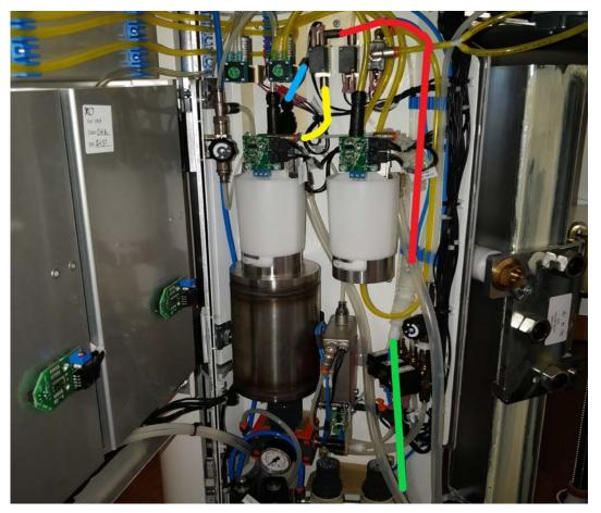
Make sure to fit the non-return valve with the arrow pointing upwards.
