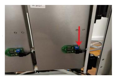
Connect cable CA-007 plug J5 to connector J5 on the backplane.
