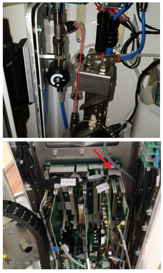
Connect cable CA-033 plug J37 to connector J37 on the Backplane. Connect the other end of the cable CA-033 plug V31 to the liquid pump V31.
