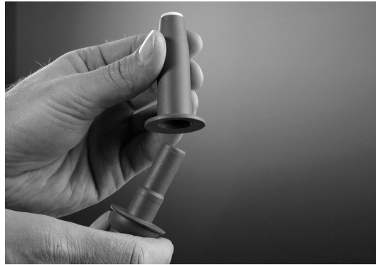
Figure 69 – Removal of suction nozzle covers
