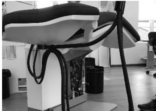
Figure 55 – Attachment of suction hoses
