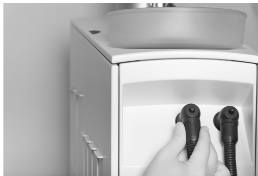
Figure 71 – Removal of suction hoses and filters
