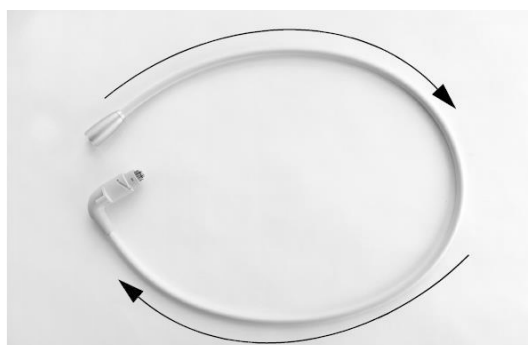
Figure 65 – Wiping direction, instrument hose-cleaning
