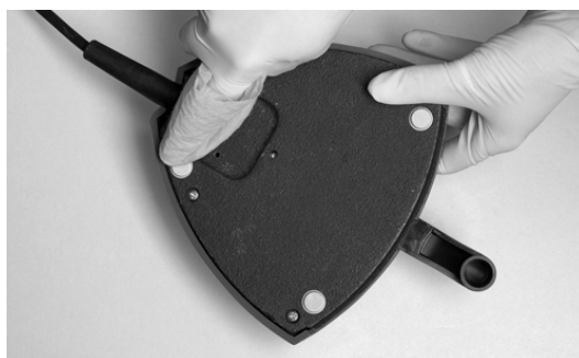
Figure 77 – Cleaning of foot control “rubber feet”
