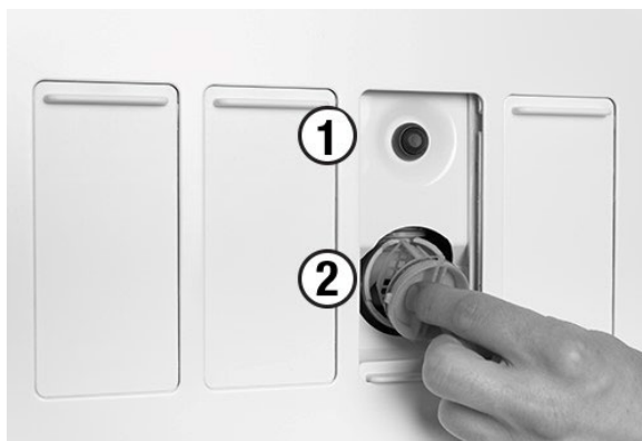
Figure 84 – Manual activation of cuspidor valve (1) and cuspidor valve filter (2)
