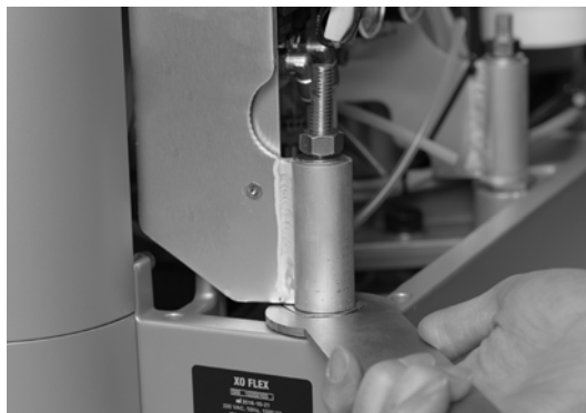
Figure 17 – Adjusting the unit base
