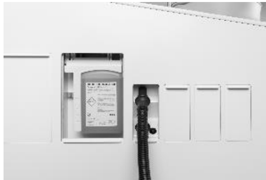
Figure 62 – XO Suction Disinfection cartridge. Note that the receiving handle is yellow.
