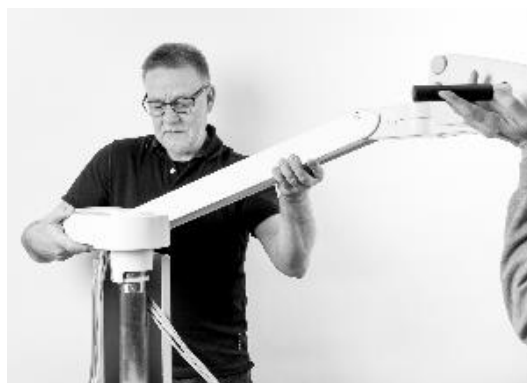
Figure 26 – Fitting the instrument bridge arm
