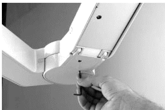
Figure 70 – Adjusting the friction brake in the swivel joint
