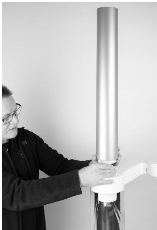
Figure 39 – Fitting the outer cylinder
