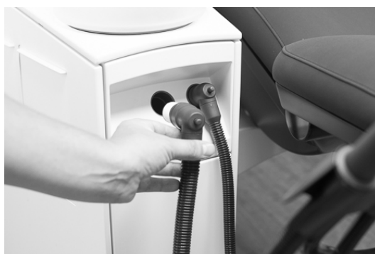
Figure 52 – Connection of suction hoses
