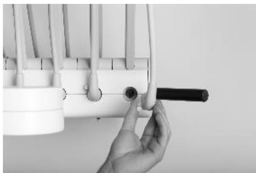
Figure 53 – Fitting the instrument suspensions and hoses
