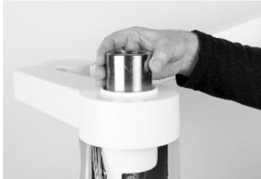
Figure 36 – Fitting the nut onto the bridge arm post
