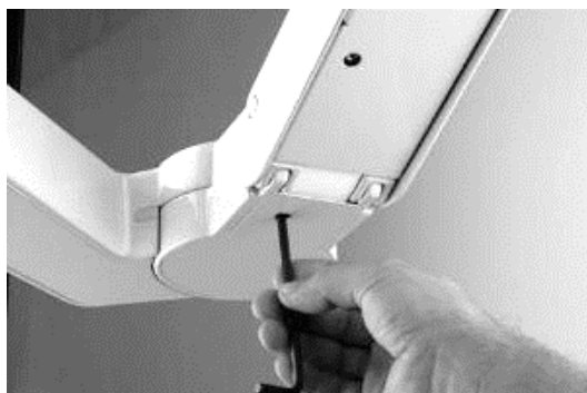
Figure 68 – Adjusting the balance spring in the bridge forearm
