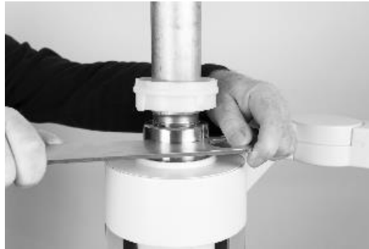
Figure 38 – Fitting the light arm post
