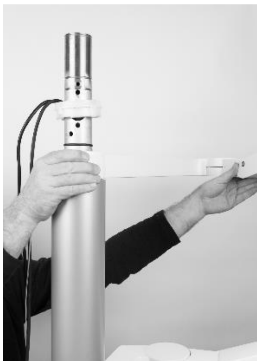
Figure 46 – Fitting of display arm
