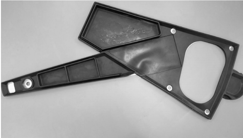
Figure 14 – Positioning of the rubber gasket
