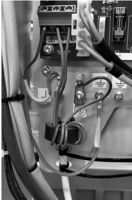
Figure 55 – Mains supply cable with ferrite
