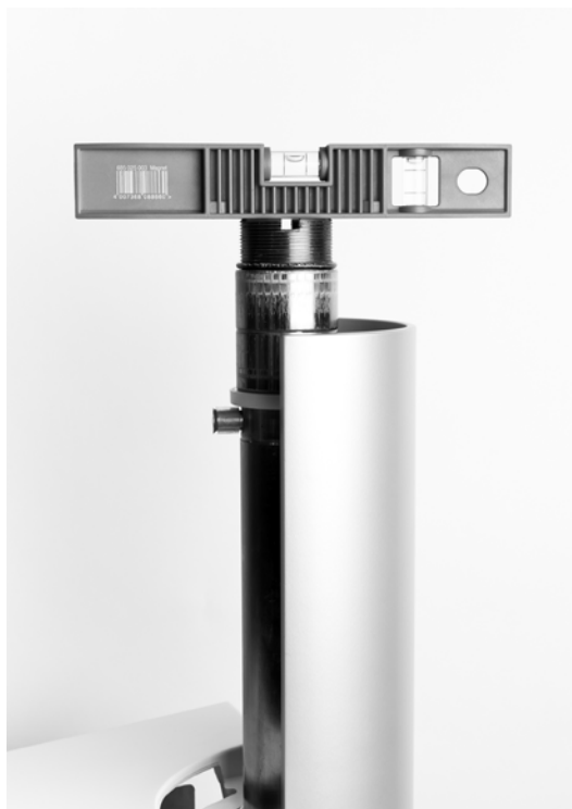
Figure 20 – Adjustment of the unit stand in longitudinal direction (A)
