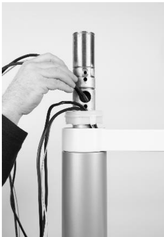
Figure 47 – Routing the display cables
