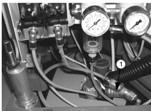
Figure 54 – Connecting incoming water and air
