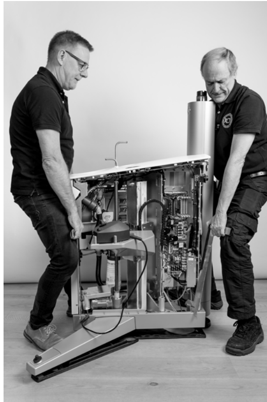
Figure 16 – Lifting the unit stand
