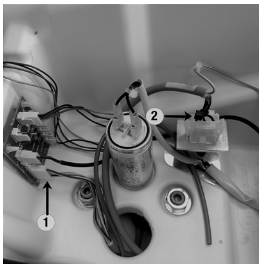
Figure 59 – Connecting the cables: (1) chair control cable, (2) chair power cable
