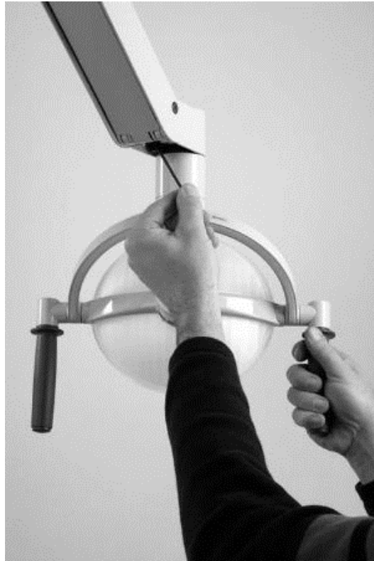
Figure 74 – Adjusting the friction in the light head
