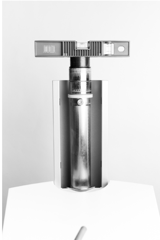
Figure 21 – Adjustment of the unit stand in the cross-wise direction (B)
