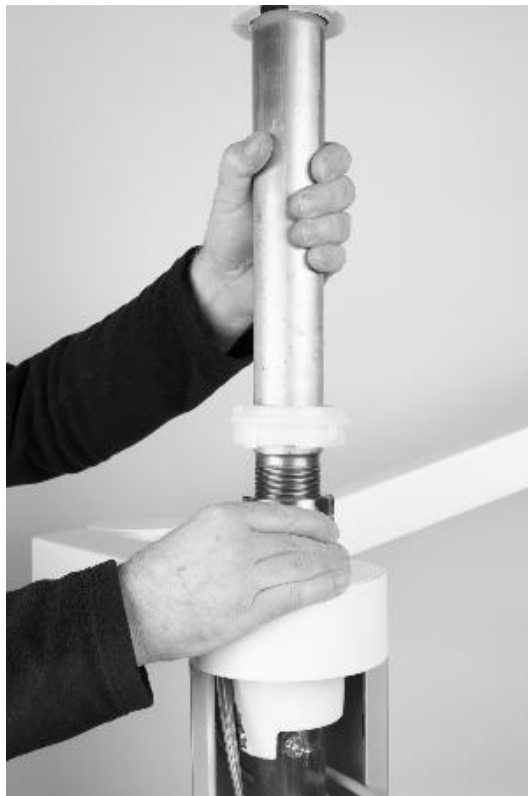
Figure 37 – Light arm post fitted into the nut
