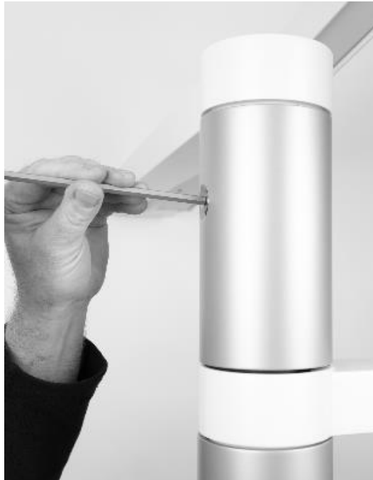
Figure 42 – Fitting the brake
