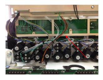
5. Install the plug on position J8 on the bridge PCB.
