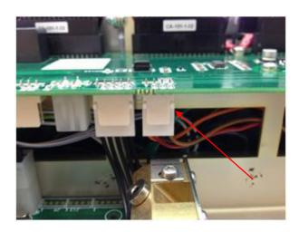
7. Close the bridge in opposite order. Make sure that all cables are in position before the screws are installed.
