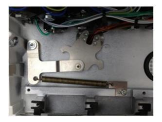
4. Install the cables from the suction holder as shown on the picture.
