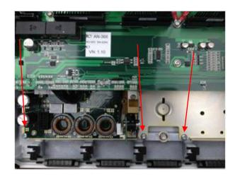
3. Install the position mechanism as shown on the picture.
