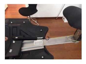
To adjust the friction, remove the neck rest from the back rest and adjust the 5 small hex key screws in the friction brake.
