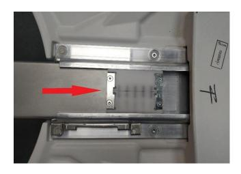
Fit the 2 nylon screws along with the neck rest stop mechanism.
