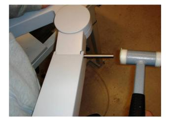
Mount the U-profile on the rear arm link1 with the axis removed previously.
