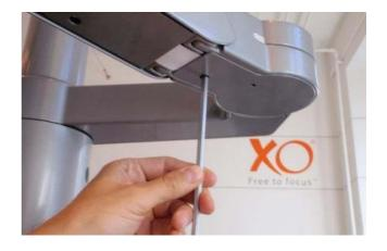
Adjust the brake (up – down) 4mm Hex tool. (Observe that it only brakes a minimum for ergonomic rear arm)
