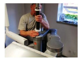
Adjust the balance force proportioned to the max weight the dentist uses with all instruments, contra angles and the tray (if used). 6mm Hex tool.
