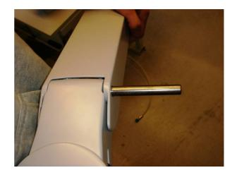
Lift up bridge to horizontal and remount the axis carefully.
