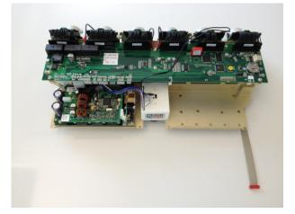
Remove the 3 upper attachment bolts in the right-hand side of the valve block rack.
