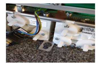
Re-assemble the block rack with the new block.
