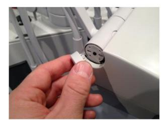
Loosen the two torx-20 bolts in the instrument bridge top cover. Remove the top cover.
