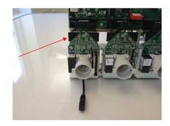
Remove the valve block from the position where you want to install the XO Odontoson 360, and install the supplied block.
