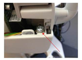
Loosen the left-hand attachment bolt for the suspension rack.
