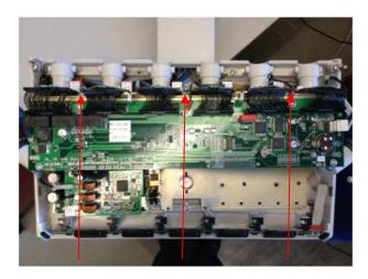
Loosen the three PCB rack attachment bolts.
