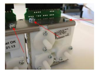
Remove the lower attachment bolt from the valve block rack.
