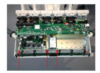
Disconnect all air, water and electric connections, and remove the PCB rack.
