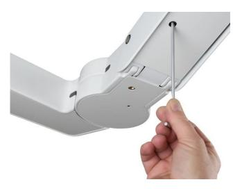
4. Move bridge arm to the top, middle and lower vertical position. The bridge arm must be able to remain in these positions, or the balance should be adjusted with a 6 mm Allen key - Verify that equal force is required to move the arm up and down.
