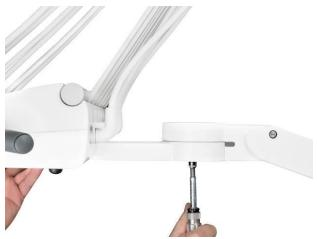
4. Check the alignment of the bearing parts before checking the center bolt.
