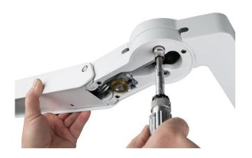
5. Check the alignment of the bearing parts before checking the center bolt.
