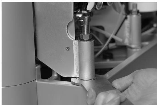
**Figure 16 – Adjusting the unit base**
