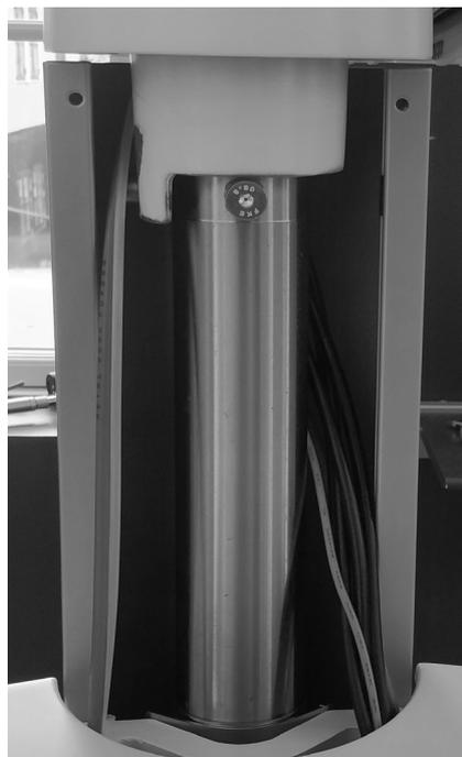
Figure 25 – Cables shall be placed between the outer cylinder and bridge arm post
