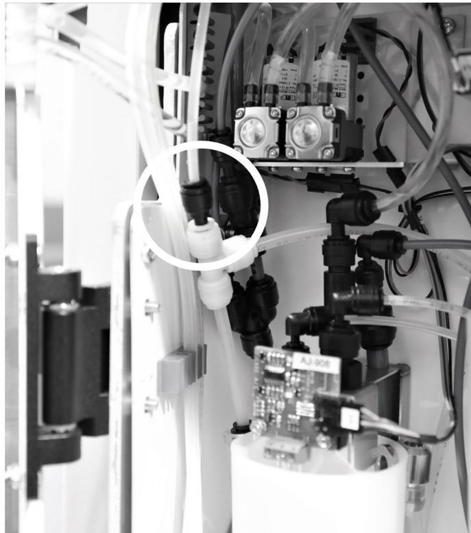
**Figure 27 – Connecting the white 4 mm water tubing from the instrument bridge to the T-fitting**
