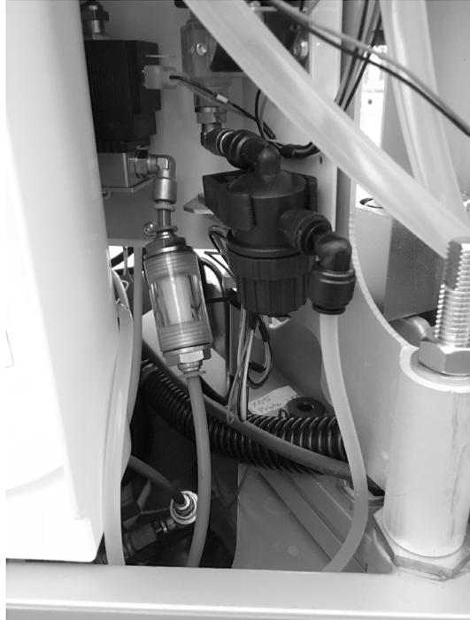
Figure 62 – Connecting incoming air and water
