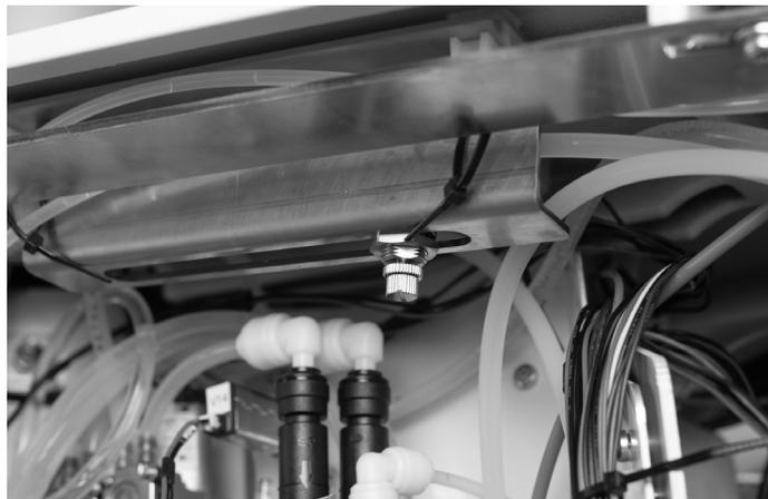
Figure 87 - Adjustment of water flow for cuspidor
