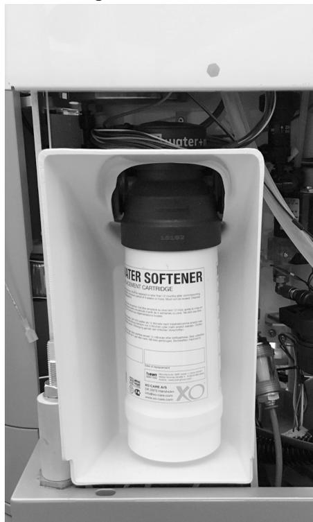
**Figure 74 – Water softener cartridge**
