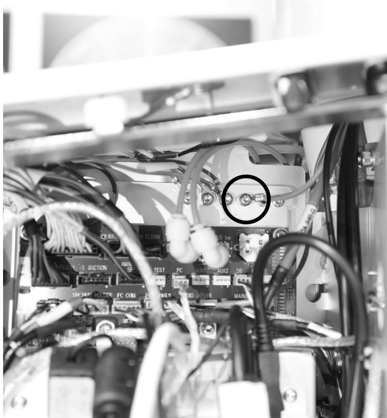
**Figure 32 - Connecting the ground cable from the dashboard**
