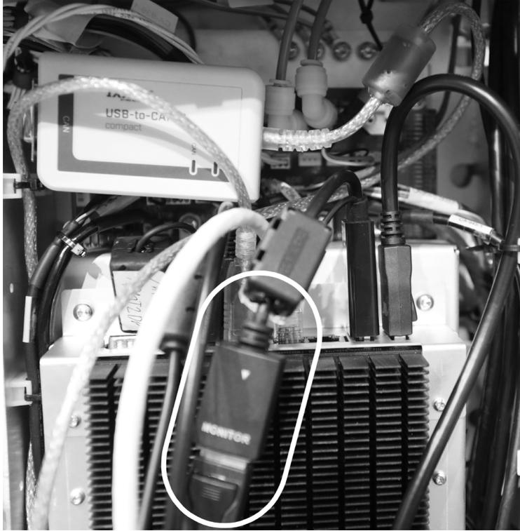
**Figure 46 - Connecting the display port cable from the Navigator to the PC**
