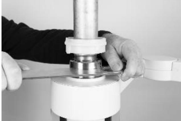
**Figure 38 – Fitting the light arm post**
