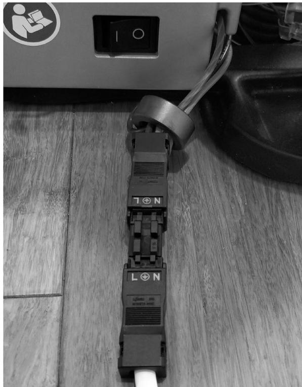
Figure 63 – Mains supply cable
