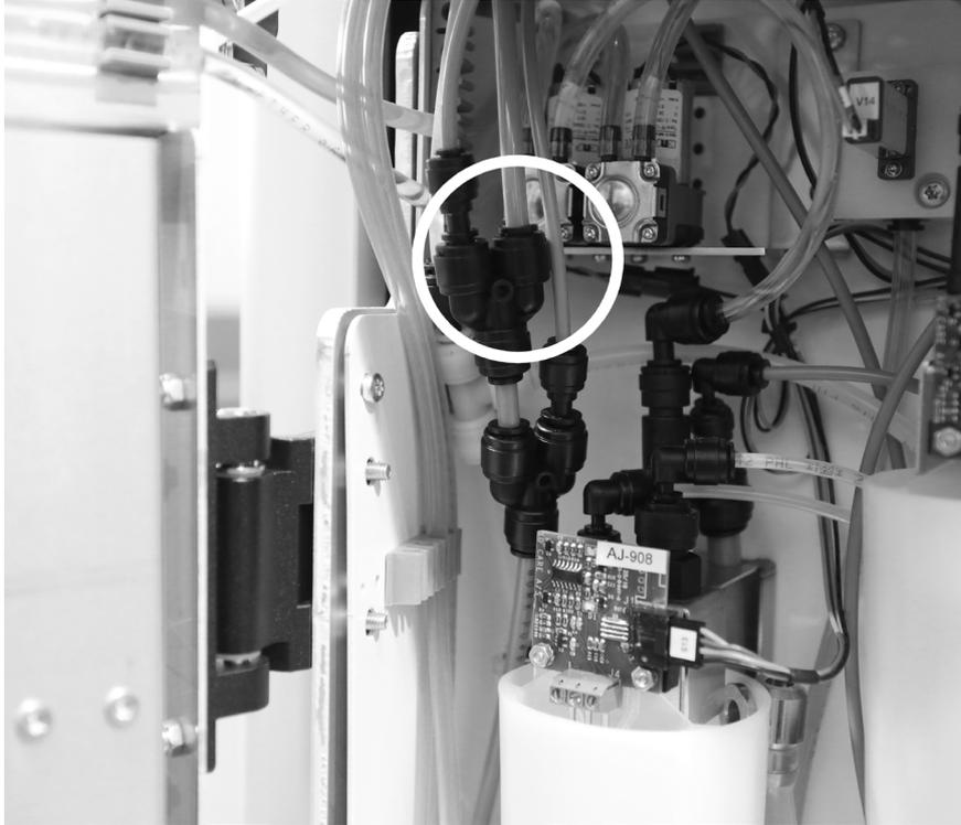
**Figure 26 – Connect the blue 6 mm air tubing from the instrument bridge to the T-fitting**
