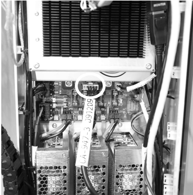
Figure 28 – Connecting cable CA-947 from the instrument bridge to BRIDGE POWER J91209
