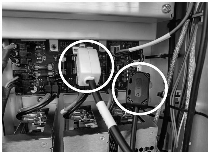
Figure 49 – Mounting the two ferrite cores onto cable CA-947 BRIDGE POWER and CA-987 Navigator communication cable
