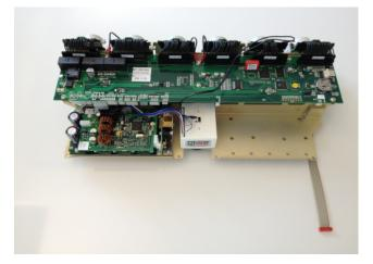
Remove as many of the upper attachment screws as needed on the right-hand side of the valve block rack, to get to the position you want to install the scaler block.
