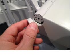
Loosen the two torx 20 screws in the instrument bridge top cover.
