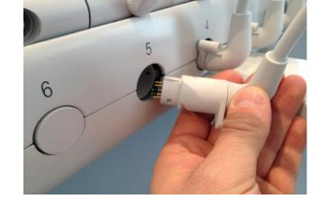
Install the Satelec scaler instrument cable in the connector in the back of the instrument bridge.
