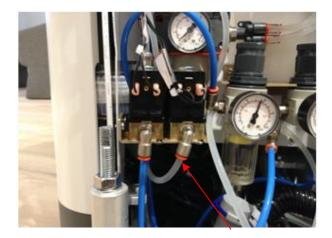
Connect the input hose from the filter to the public water supply fitting.
