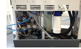
The drain hose(s) should be routed under the filter cartridge.
