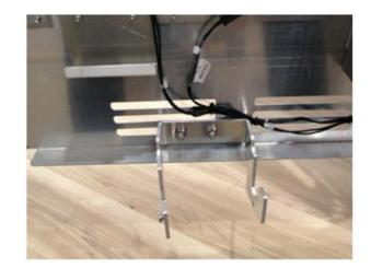
Attach the bracket with the bolts.
