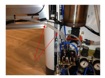
Connect the outlet tube from the filter, to the inlet on the main water valve.
