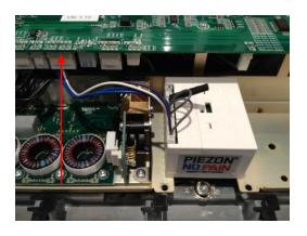
9. Install the EMS module attachment torx 10 bolts.
