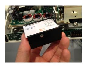
8. Install the EMS No pain scaler module. Connect the network to receptacle J5 on the bridge PCB.
