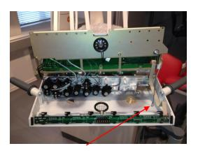
5. Remove the loudspeaker. The loudspeaker is attached with adhesive foam.
