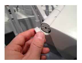
2. Loosen the two torx 20 bolts in the instrument bridge top cover.
