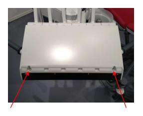
3. Loosen the 3 torx 20 bolts in the electronic bridge rack.
