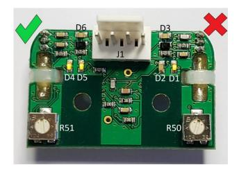
When the four LEDs are equally bright, switch the unit off.
