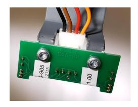
Reconnect the cable to the new PCB (AP-297 / AD-634) and fit the new PCB with the same two screws.
