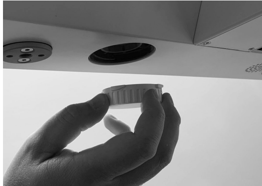
Figure 70 – Accessing the oil separator
