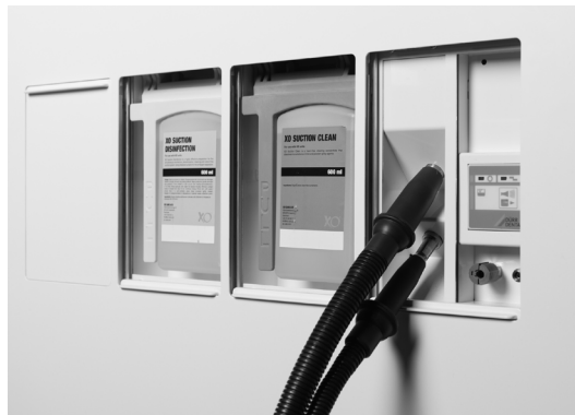
Figure 63 – Suction hoses ready for disinfection of suction system
