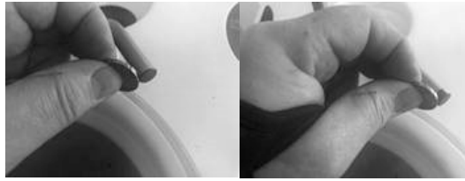
Figure 80 – Removal of spout nozzle
