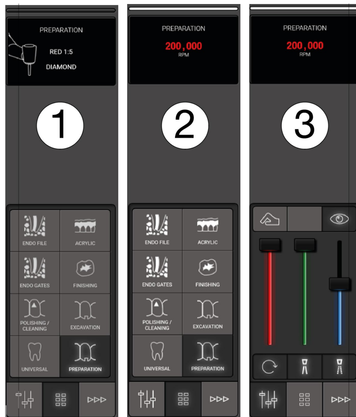
Figure 19 – Preset: (1) Preset activated, (2) instrument activated and (3) monitoring and adjustment of preset
