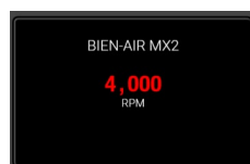
Figure 12 – Instrument display showing the actual micromotor speed
