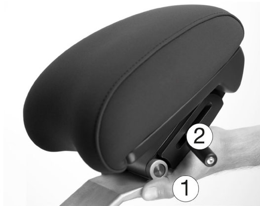
Figure 34 – Neck rest: (1) push the neck rest while the chair moves and (2) release handle
