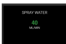
Figure 14 – Instrument display: Monitoring and adjustment of amount of spray water
