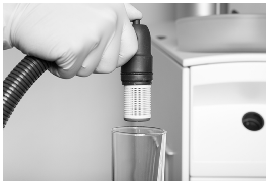
Figure 89 – Press the button to eject the filter holder and cartridge
