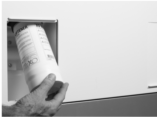
Figure 94 – Replacing the water softener cartridge
