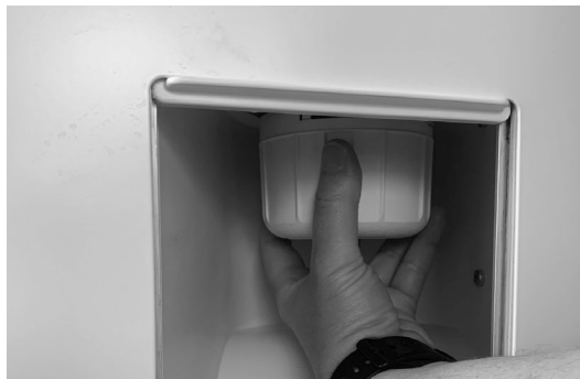
Figure 93 – Replacing the amalgam collector vessel
