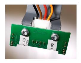
Fit the new PCB (AD-633 / AO-989) with the same two screws and re-connect.
