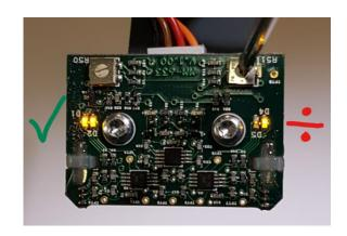
When the four LEDs are equally bright, switch the unit off.
